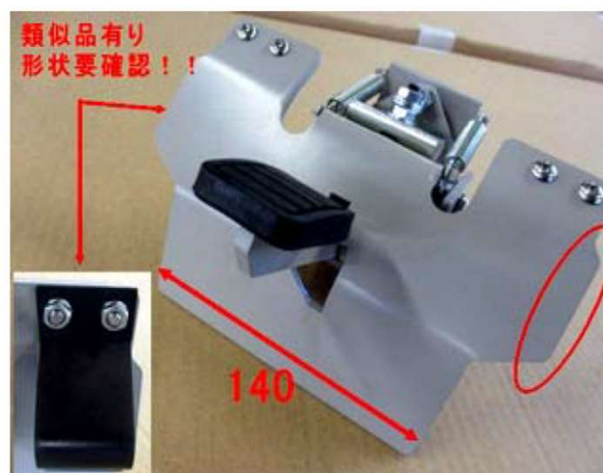
BM8-2 Parking Brake with Foot Guard
